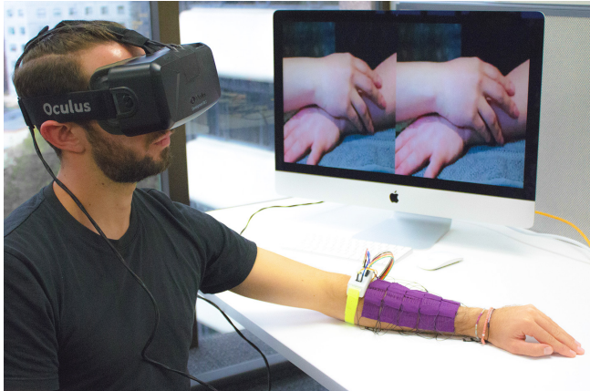
Figure 3. We recreate the perception of a human touch using plasters that stimulate the skin with shear forces. Here, the user is experiencing the touch of another's hand on his arm.
