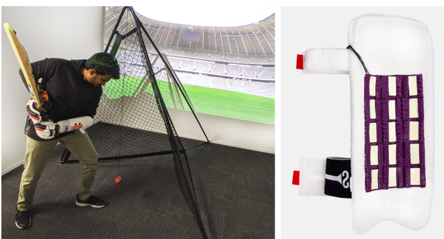
Figure 15. A participant receives guiding feedback via an arm-guard, augmented to receive natural touch sensations.
