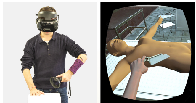
Figure 16. A participant interacts with a medical-surgical training simulation, enhanced with additional feedback provided on the forearm.
