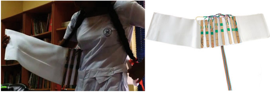
Fig. 10 Participant wearing the VibroBelt. The prototype consists of 8 stripes with attached vibrator motors
