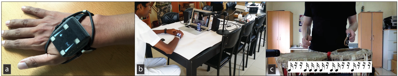
Figure 3. The setup and stimuli of the controlled user study: (a) MuSS-Bits was attached to the palm, (b) in light condition an additional Display-Bit was close to the screen, and (c) the participants could see the scores for the reproduction task.
