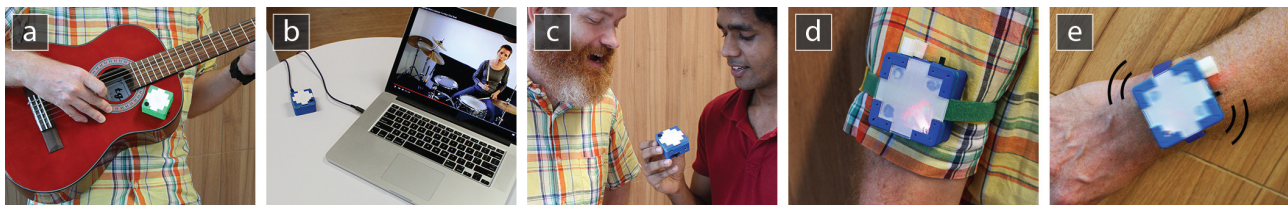
Figure 1. MuSS-Bits sense sound from (a) an instrument, (b) a digital device, or (c) the environment and translate it to (d) visual and (e) vibrotactile feedback.
