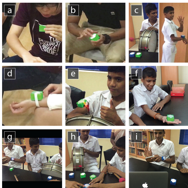
Figure 5. Deaf users interacting with MuSS-Bits: (a) blowing into microphone; (b) tapping on Sensor-Bit surface (c) participants playing a counting game; (d) Display-Bit worn around the wrist, (e) the upper arm and (f) held on the hand; (g) collaborative music-making; (h) sharing of a Display-Bit; (i) following an online tutorial.
