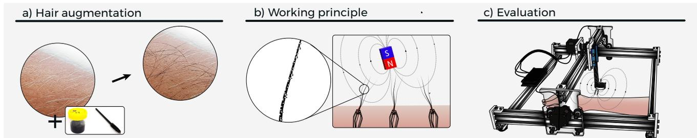
Figure 1. a) Forearm Hair of participant after applying passive magnetic cosmetics. b) The hairs are attracted by the magnetic fields providing tactile feedback. c) Setup of the evaluation with a CNC engraver (wooden enclosure not shown)
