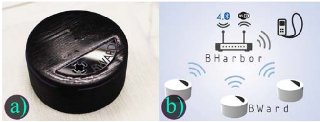
Figure 2. a) BWARD prototype placed over a clean dressing b) System overview.
