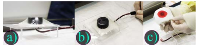
Figure 9. a) BWARD testing real blood set up b) Real blood being injected in the dressing c) Dressing after detection positive blood detection
